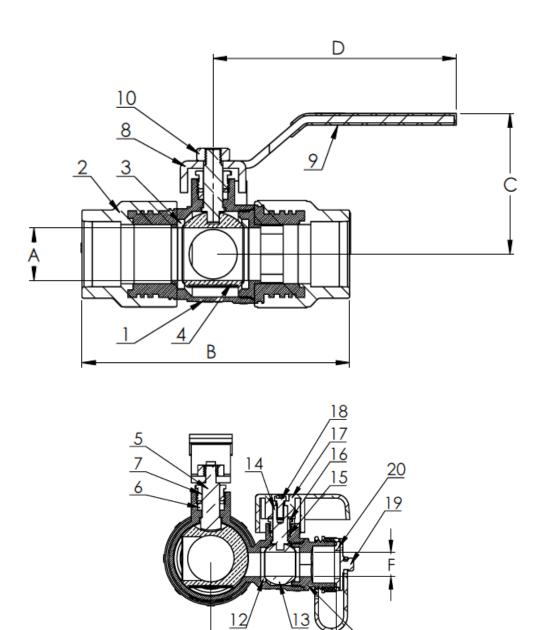
**Specifications:** Designed for residential, commercial or industrial use with water, oil or gas. This approved Webstone valve is actuated by a blowout proof stem and features an adjustable packing gland. Socket end dimensions are in accordance with ASTM F 2389 Metric Series.
